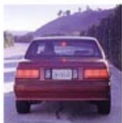
Hologram, developed by Hughes and Inland Fisher Guide, projects brake light on a car's rear window, but remains invisible to the driver.
