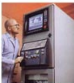
Machine tool controllers enable operators to program factory equipment for increased productivity and precision.
